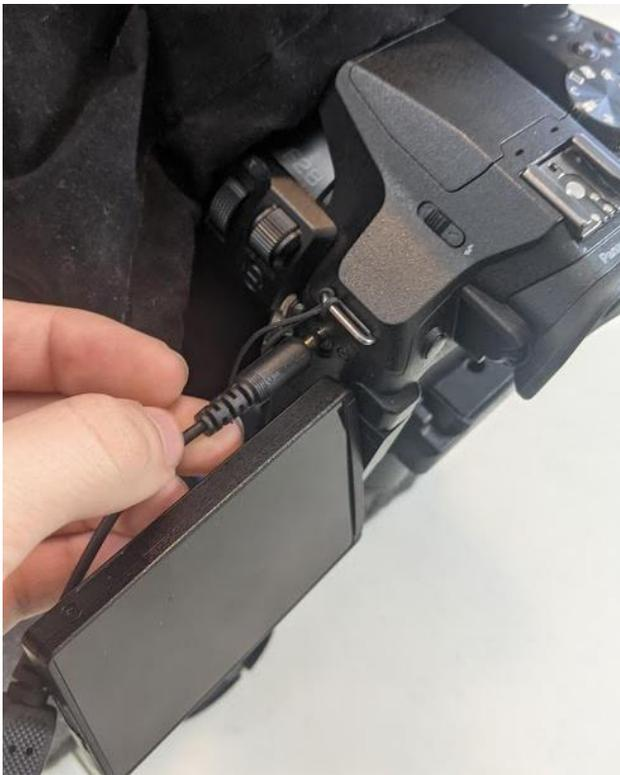
2. Turn on the camera (pink circle) by moving the switch to on. Set the camera to video recording mode for best results (red circle) by turning the dial. Then when aiming the camera at the subject, push the red record button to record video (blue). To stop recording, push the record again.
